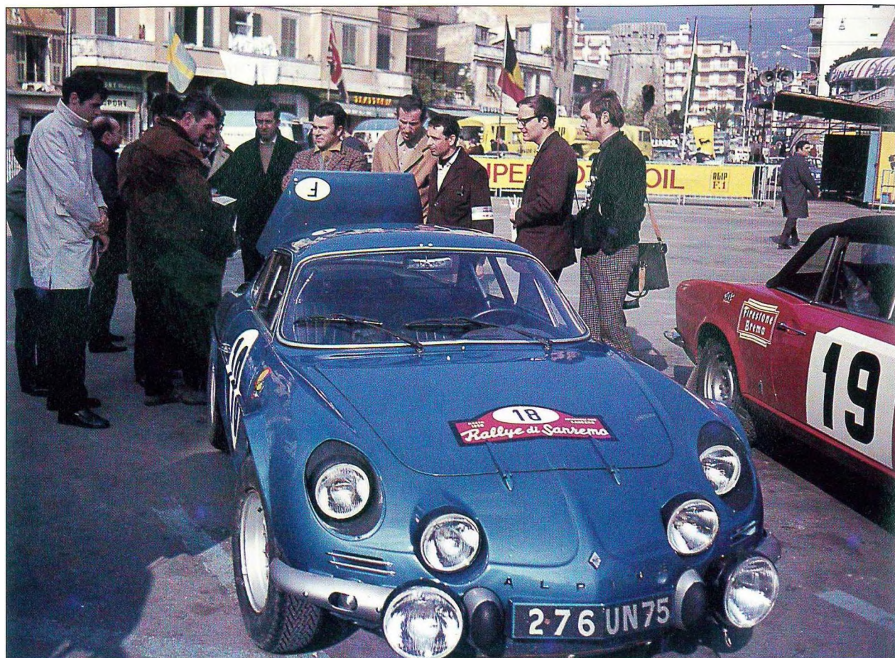
ABOVE The classic features of a classic rally car – the Alpine A110 was underpowered in its early years and rather unreliable, but once it discovered the 1600cc Renault engine and the suspension was properly developed, it became a winner everywhere but the Safari and the RAC Rally.
